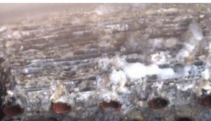
Unprotected coil after 4000 hours acid spray test
